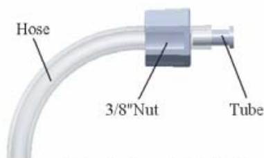
Figure 7 Installation of Acid-alkaline Drawing Pipeline
